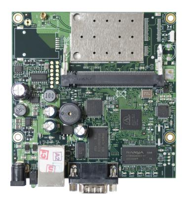
The RB411AR is has a built-in 802.11 b/g wireless card with a sturdy MMCX connector, and a spare miniPCI slot for another wireless card.
