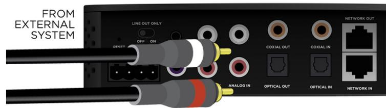
1. Connect the external audio source to the analog, optical, or digital input.
