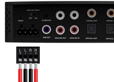
2. Connect the phoenix connector, auxiliary audio sources, and external audio subsystems.
