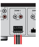
2. Connect all phoenix connectors, auxiliary audio sources, and external audio subsystems.
