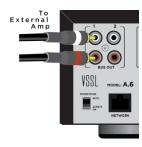
**Note:** The A.6 outputs should only be connected to another amplifier system and not a system that redistributes the signal, such as an audio matrix. Doing so may cause unintended consequences and cannot be guaranteed.
