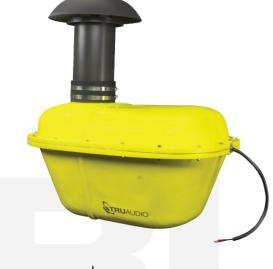
Speaker Type: Woofer: Power: Impedance: 70v Taps: Freq Response: Sensitivity: Enclosure: Finish Dims: Underground Subwoofer 12" injected polypropylene 400 watts 4 $\Omega$  or 70V 200W 28 - 90k Hz (+/- 3dB) 89 dB Fiberglass reinforced plastic 24.7" (624mm) L, 21.6" (548mm) W, 33.7" (855mm) w/port
