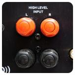
To connect your subwoofer using the "High Level Input", connect a quality speaker cable from the left and right speaker outputs on you're a/V processor to the left and right inputs on the back of the subwoofer. Please
