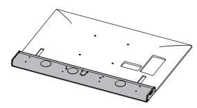
2) To determine which Vertical Bars to use, place a bar even with the edge of the TV where the soundbar will be mounted. The slot in the bar should cover both VESA holes, but not extend beyond the TV.
