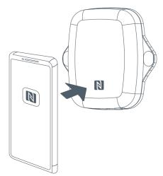
4. Basic information and settings of devices will be shown on ToolBox if it's recognized successfully. You can turn on/off the device by tapping the button on the Device Status. In order to protect the security of devices, password validation is required when configuring via unused phone. Default password is **123456**.
